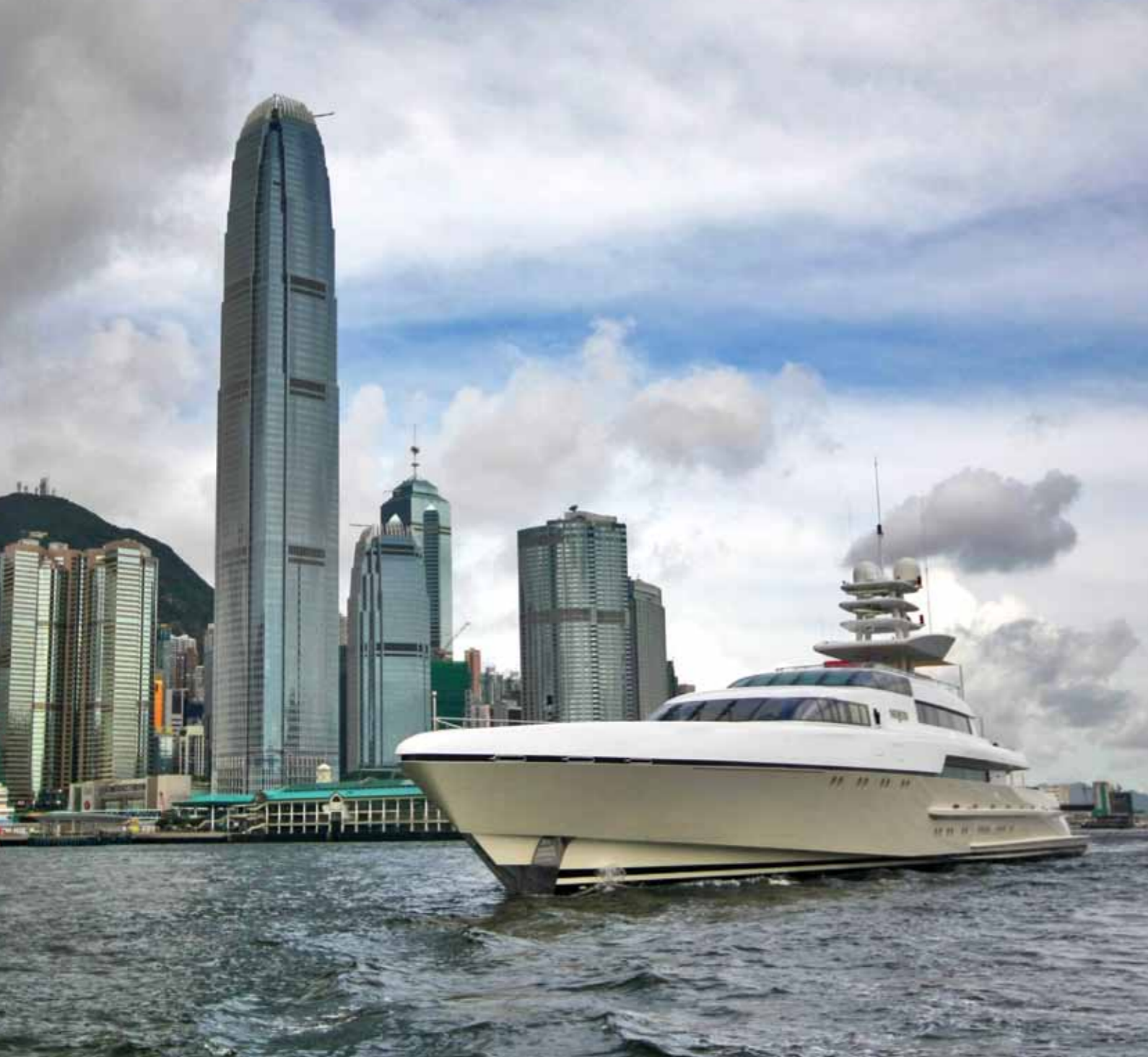
Silver Zwei covered the distance between Abu Dhabi and Singapore in 12 days, averaging 20 knots at 400 litres/hour.
